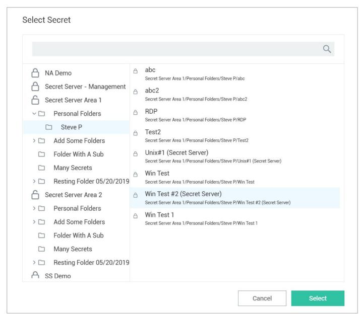
The Select Secret dialog box shows the currently existing connections. Those that are authenticated and accessible, are shown with an open lock next to the name. A closed lock indicated authentication is required, generally a username and password. Users can drill-down the navigation tree to access more folders.
